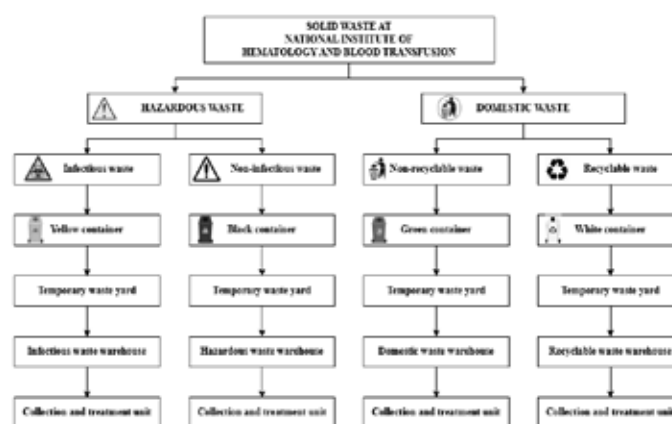
Figure 1. Solid waste collection diagram at NIHBT
