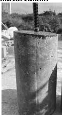
a) Plain Concrete Sample
